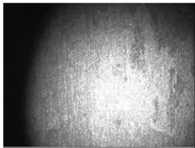
Fig. 3. Cerium-containing coating obtained by deposition during 20 s (optical microscope).
